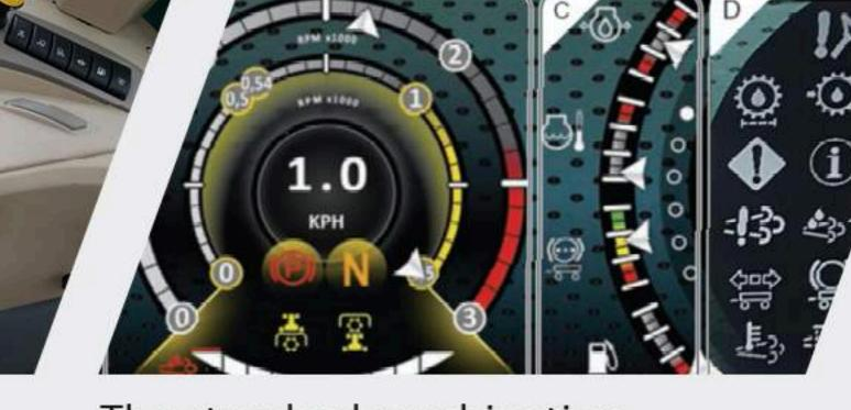
The standard combination instrument panel has been upgraded to a multifunctional LCD dashboard that can display fault codes.
