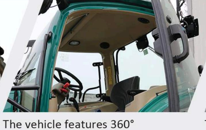
The use of a combination switch panoramic curved glass and a fully and the concentration of most of enclosed cab with four pillars and the operating handles in the rightair conditioner, providing a wide hand area have greatly improved ergonomics.
